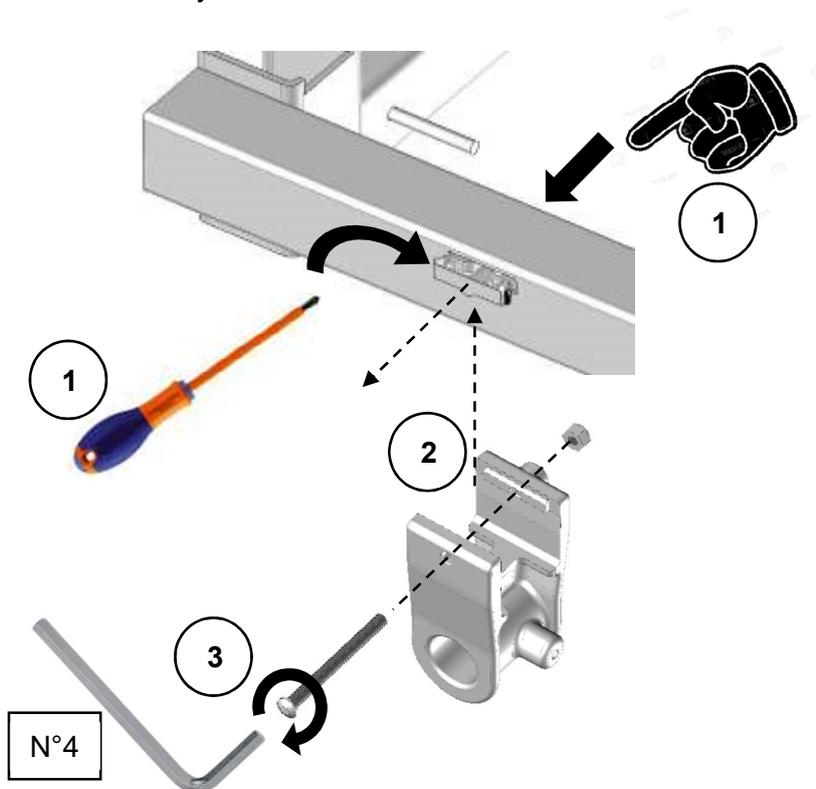
① Remove the cap of the siderail by pushing inside or outside (depending on the assembly) then remove it with a screwdriver if necessary.
