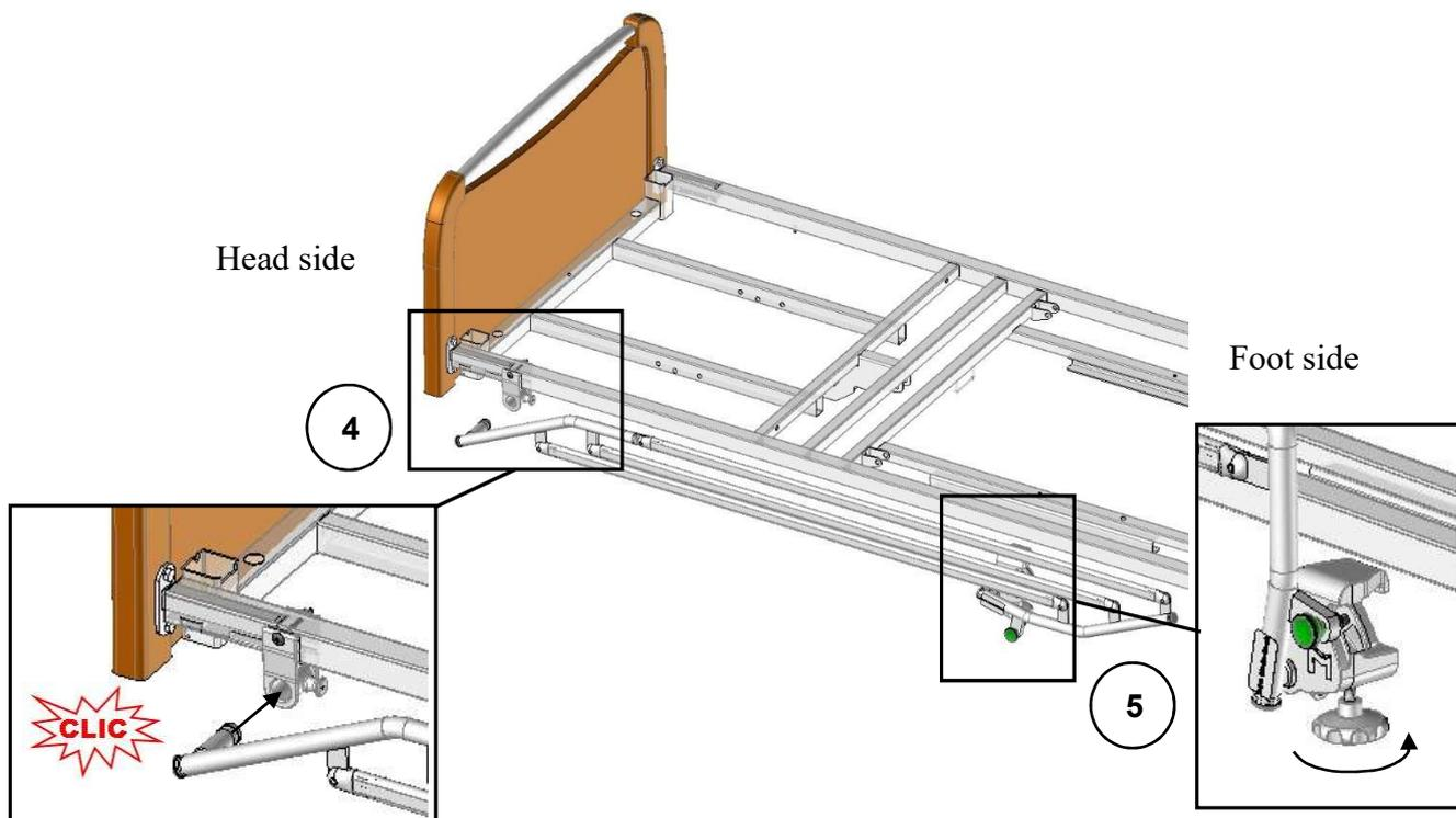
④ Insert pole of the side rail in the jaw on the head side fixed on the bed until to hear the «CLIC».
