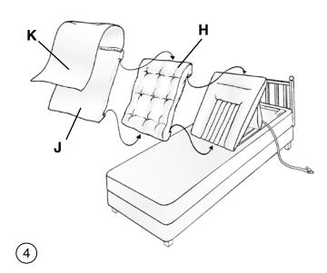
Position your pillow on the Handy Pillow Lift as indicated (fig. 5) and wrap the flap (K) completely around the pillow to hold it in place.
