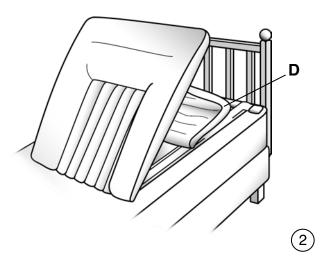
Remove the pillows from the bed and place the Handy Pillow Lift on the bed with the Spreader Bar positioned up against the headboard. Fold the strut (**D** fig.2) towards the headboard.
